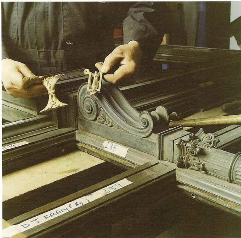
These replica castings before toning, contrast against dirty cast screens showing the early stages of green patination, before cleaning and refinishing.
